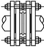
"MAXIMUM TRAVEL" (±) MAY BE CALLED LONGITUDINAL MOVEMENT OR AXIAL COMPRESSION AND EXTENSION. IT IS BASED ON INSTALLATION WITH NO MISALIGNMENT OR ANGULAR DEFLECTION.
