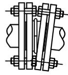
"MAXIMUM ANGULAR DEFLECTION" MAY BE CALLED ANGULAR ROTATION. IT IS BASED ON INSTALLATION WITH NO AXIAL TRAVEL OR LATERAL OFFSET.
