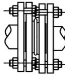
"MAXIMUM MISALIGNMENT" MAY ALSO BE REFERRED TO AS LATERAL OFFSET OR DEFLECTION. IT IS BASED ON INSTALLATION WITH AXIAL TRAVEL OR ANGULAR DEFLECTION.
